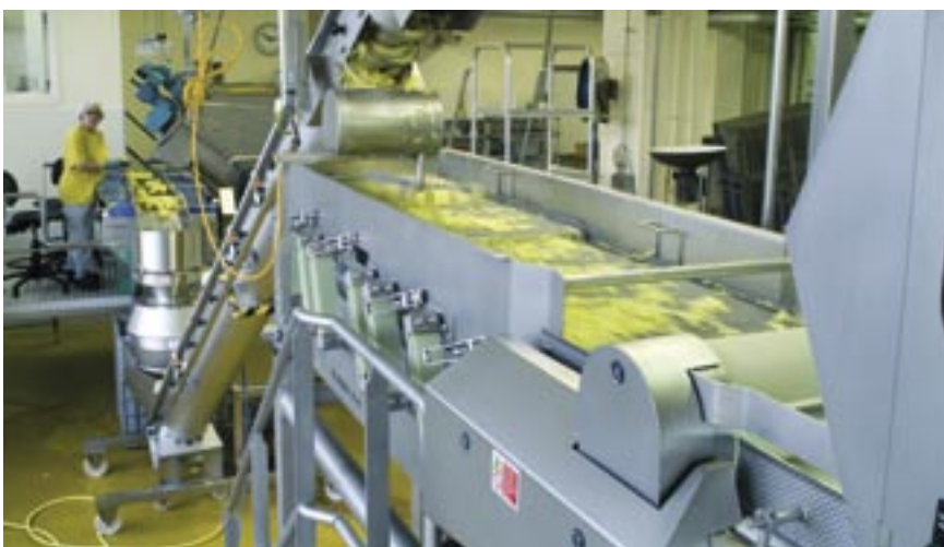
Infeed of shredded potato
