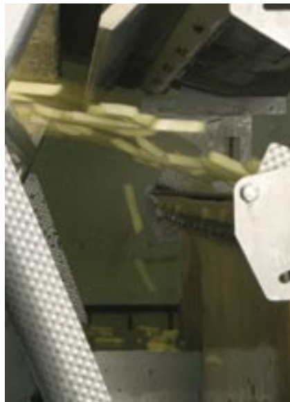
Optyx ejector system on potato strip line
