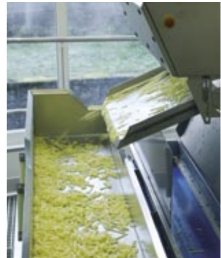
Discharge from Optyx on shredded potato line
