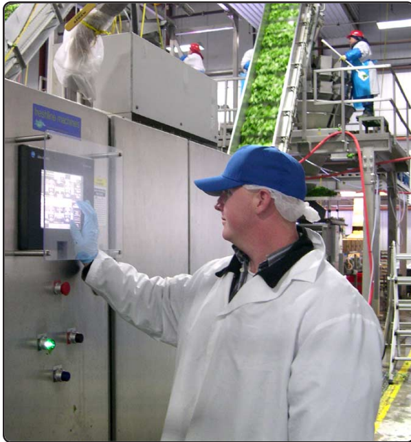
True Leaf Farms system operator selects a new recipe to switch between product batch types on Key's ADR980 Automatic Dryer.
