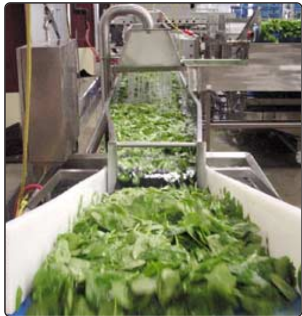
True Leaf Farms spinach transfers from the second stage DirectStream washing to drying.
