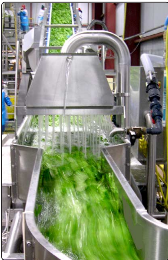
Key's DirectStream meters and gently washes tender leaf product in a continuous flow process at True Leaf Farms.
