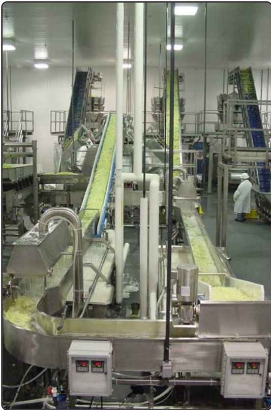
Typical installation processing lettuce
