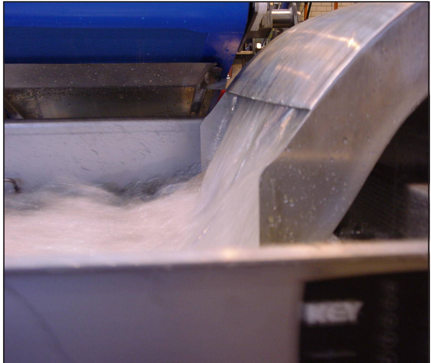
Water Delivered to Shaker Wash
