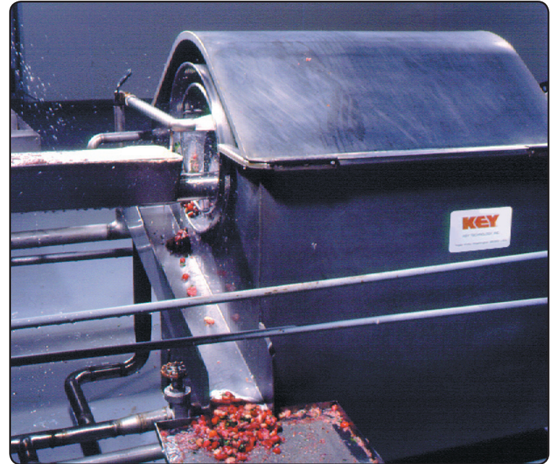
Reclaim Reel on a Strawberry Processing Line
